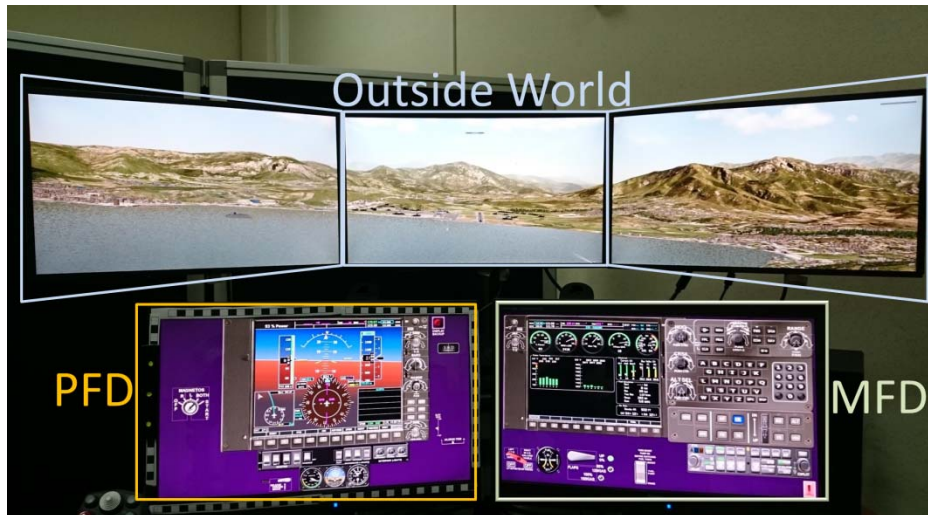
Fig. 1. Cirrus Perspective with Garmin 1000 simulator environment (CReA)
