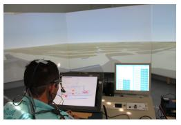
Figure 3. Experimentation on our simulator. Participant face (top to bottom, left to right) out-the-window view, radar screen, flight list and stripboard. Neurophysical data such as eyetracking, electroencephalography, and electrocardiography are recorded.
