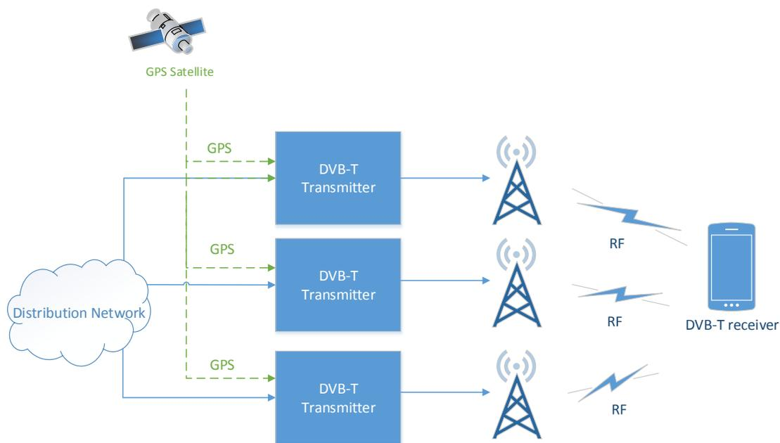
Fig. 1. DVB-T SFN transmission
