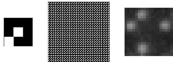
**Figure 3: The displayed texture (middle) is composed of a repetition of the 3×3 pixels pattern composed of black and white pixels (left). Image of the texture captured by the ADNS-2610 mouse sensor (right) showing the screen door effect is canceled.**
