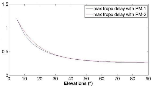
Figure 10 -  $\mu_{max}$  with the 2 new methodologies
