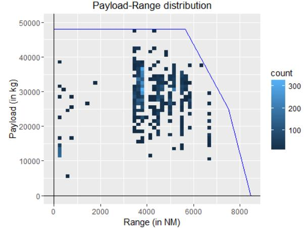
*Figure 9. Payload-Range distribution*
