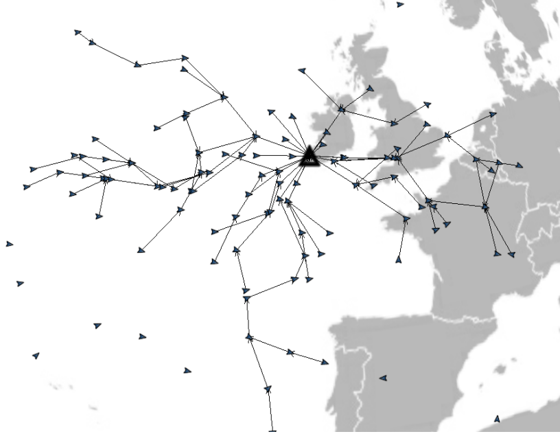
Figure 2: Routes toward a single ground station obtained with AODV in an AANET (the ground station is figured by a black triangle).
