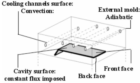
Figure 1: Boundary conditions applied on the mould
