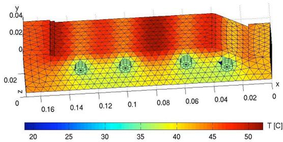
Figure 4 : Optimised position of the cooling channels.
