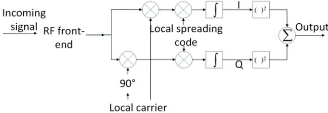
Fig. 1: Block diagram of the serial search acquisition
