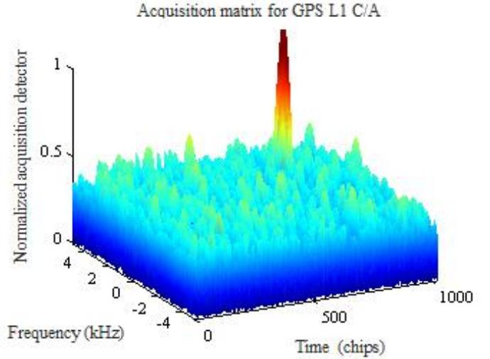
Fig. 2: Acquisition matrix output from serial search acquisition
