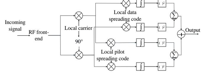
Fig. 10: Conceptual scheme of the data/pilot signal acquisition
