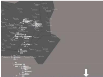
Figure 7. SmartPan: the arrow indicates a calling aircraft outside the radar image.
