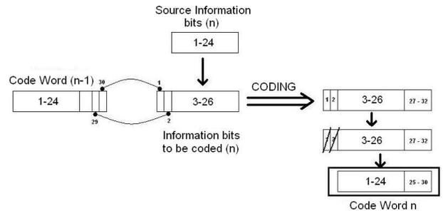
Figure 3 – GPS L1 C/A signal PC encoding process
