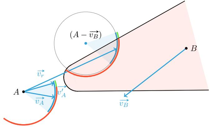
Figure 2. Possible headings for conflict avoidance: the end of  $\vec{v}'_r$  must lie on the circle but outside of the forbidden zone (in light red) and in the allowed turn angle range of  $\pm\theta$  ( $\theta = 30^\circ$ ) around  $\vec{v}_A$ , which leaves the tiny green safe zone as possible new heading for the UAS.
