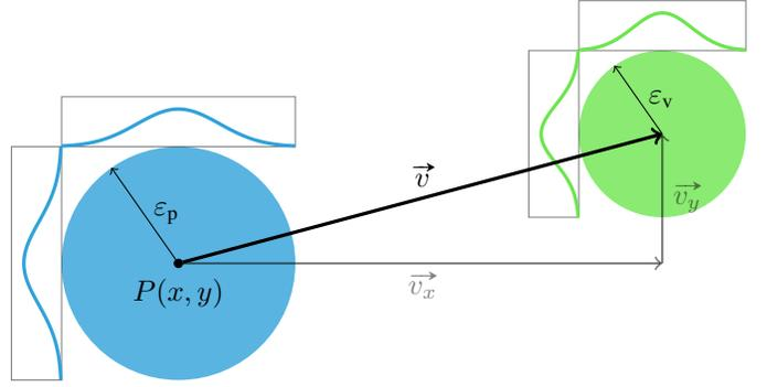
Figure 4. Modeling of accuracy:  $\epsilon_p$  (resp.  $\epsilon_v$ ) represents the 95% accuracy bound for the position (resp. velocity) of UAS and aircraft. Each component of the position (resp. velocity) follows a normal distribution.
