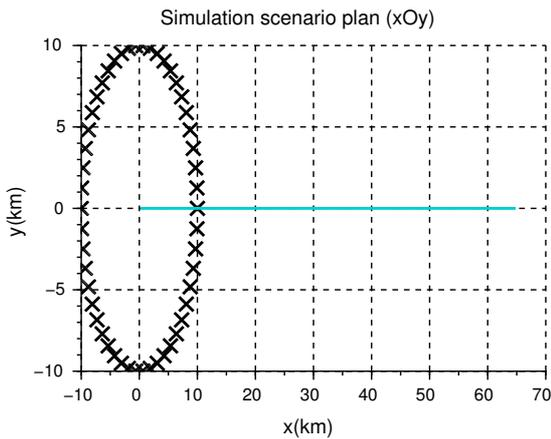
Fig. 1. Geometry of the first test case. The VOR station is at the origin. The crosses represent wind turbines. The blue line is the trajectory chosen for the simulation.
