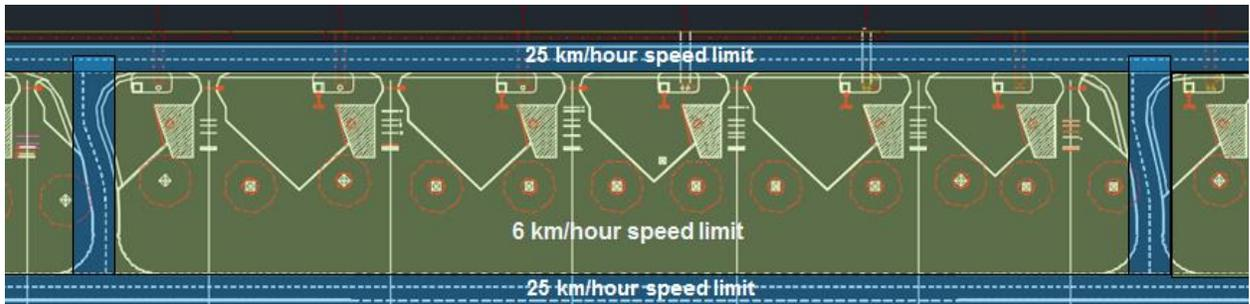
Figure 6: Typical airport parking layout showing speed limits by zones. Source: authors
