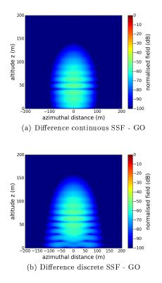
Figure 5: Propagation of a 3D complex source point over an impedance ground.
