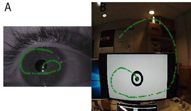
Figure 16: Recorded pupil location (in the pupil camera) on the left, corresponding target position on the right. Similarly, EyeRecToo (Santini, 2017) proposes an innovative way to collect such calibration points using a marker on a mobile phone.
