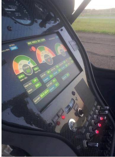
Fig. 8. The Volta cockpit HMI
