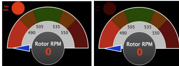
Fig. 9. The two graphical states of the blinking “low RPM” alarm
