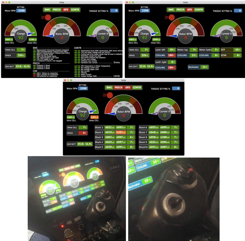
Fig. 11. The three pages of the Volta HMI, and the left-right switch on the joystick to navigate them. The switch is connected to two GPIOs on the embedded platform.
