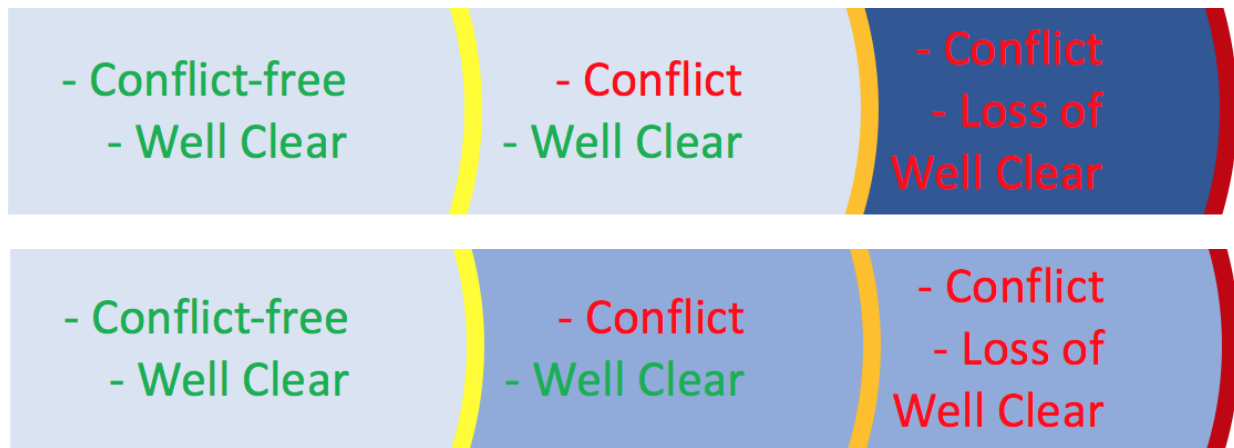
Figure 2: Two boundaries (yellow, orange) separate the different states. Top, the ownship does not have the right of way. Bottom, the ownship does have the right of way. As an encounter evolves, the ownship possible manoeuvres are increasingly constrained: none (clear), maintain heading and speed (darker), constrained according to Right of Way rules (darkest).
