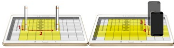
Figure 4: Intersection technique: stack (1) and translation (2) to select columns and stack (3) and translation (4) to select rows.
