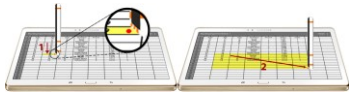
Figure 5: Stack and Drag technique: stack of the smartphone (1) and translation (2) to extend the selection.
