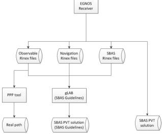
Figure 4 – Data process scheme
