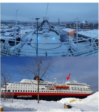
Figure 3 – Antenna position in MS Finnmarken
