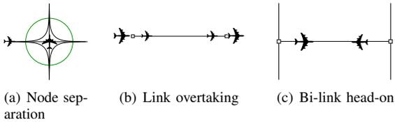
Fig. 4: Taxi separation based on node-link network.
