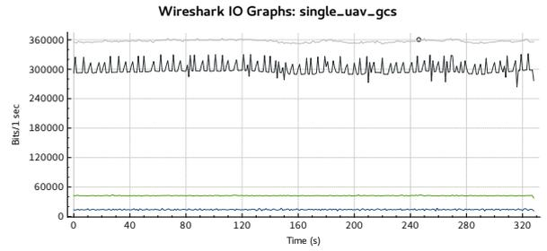
Figure 7. Traffic characterization (from the lowest to highest: telemetry, C2, video, moving average of total data)
