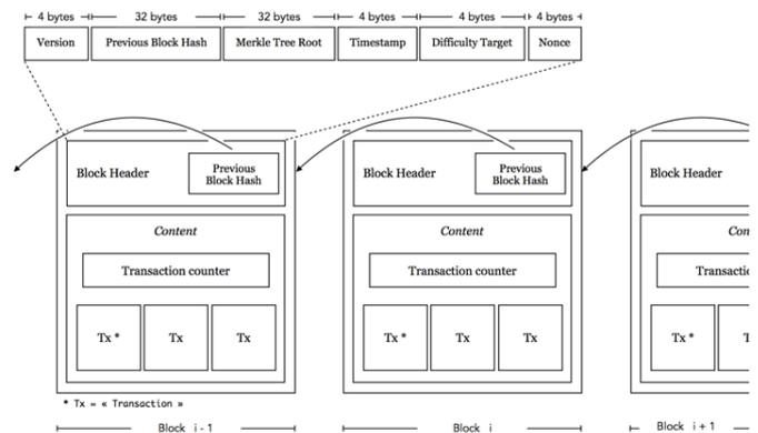
Figure 1 - Simplistic view of a Blockchain's data structure [13]
