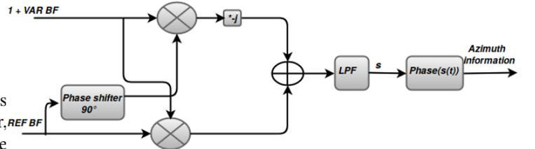
Fig. 4: Block diagram of the phase detector.
