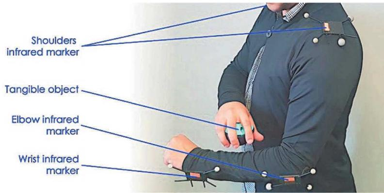
**Fig. 2.** Placement of the infrared tracking markers
