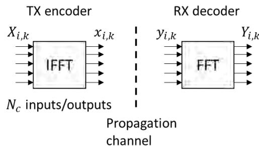
**Figure 1.** OFDM encoding and decoding blocks. Notation:  $X_{i,k}$ , TX data symbols;  $x_{i,k}$ , TX OFDM symbols;  $y_{i,k}$ , RX OFDM symbols;  $Y_{i,k}$ , RX data symbols. The letters  $i$  and  $k$  represent the OFDM symbol index and the subcarrier index, respectively.
