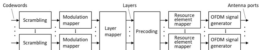
**Figure 3.** LTE downlink physical channel processing chain
