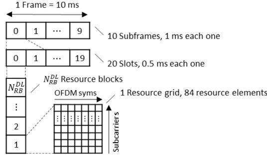
**Figure 2.** LTE frame structure. Abbreviation: syms, symbols
