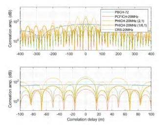
**Figure 12.** Autocorrelation amplitude as a function of the correlation delay for a set of different physical channels within a common signal of 20 MHz channel bandwidth; (top) zoom out (bottom) zoom in. Notations: PHICH-20MHz (2,1), denotes PHICH for channel bandwidth 20 MHz, for  $N_g$ = 2 and for a single orthogonal sequence per PBCH group; PHICH-20MHz (1/6,1), denotes PHICH for channel bandwidth 20 MHz, for  $N_g$ = 1/6 and for a single orthogonal sequence per PBCH group
