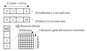
Figure 2. LTE frame structure. Abbreviation: syms, symbols
