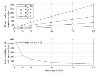
Figure 11. PHICH autocorrelation amplitude (top) maximum (bottom) main lobe width as a function of the number of resource blocks for a different setting of the PHICH resource indicator  $N_q$
