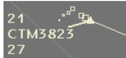
Figure 1 : the ODS comet of an evolving aircraft, the image exhibits direction and acceleration changes
