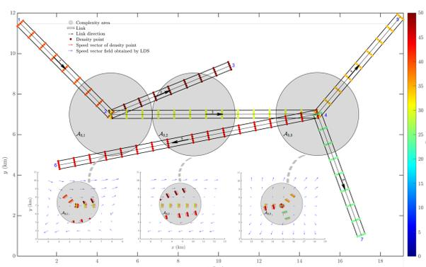
Figure 3: Illustration of density points on grids, discal complexity evaluation areas, and vector field of LDS
