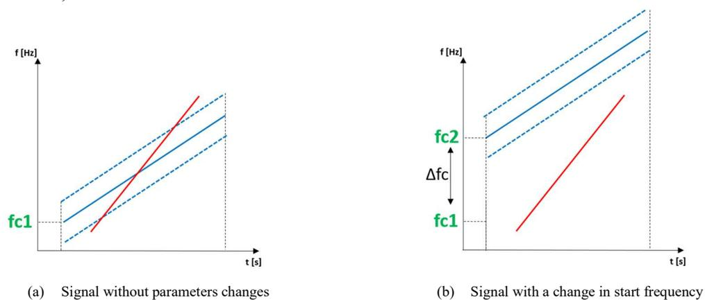
**Figure 6 – Example of start frequency change to avoid interference**
