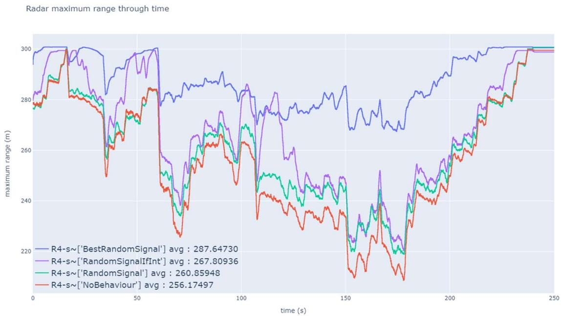
**Figure A2 – Average max range for radars on a 3km highway, 10 vehicles simulation**
