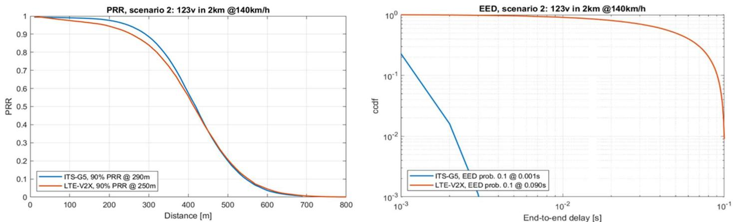
Figure 4 – V2X reference PRR and EED curves for ITS-G5 and LTE-V2X
