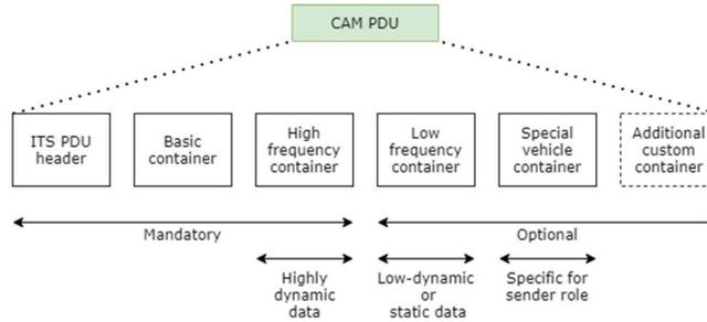
Figure 1 – CAM payload
