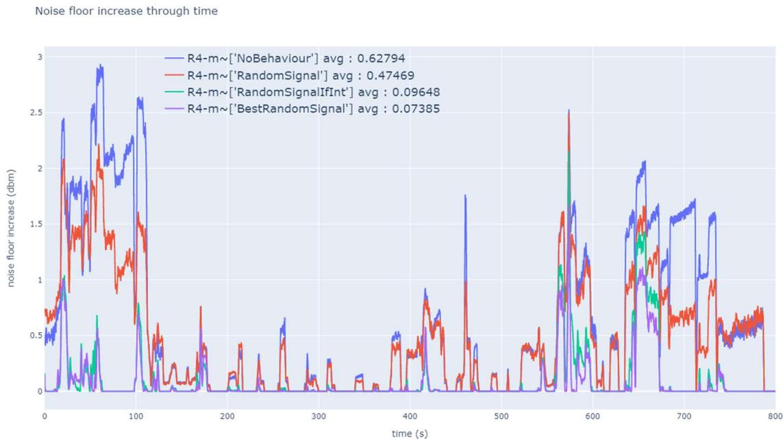
Figure A3 – Average noise floor increase for radars on an urban layout, 10 vehicles simulation
