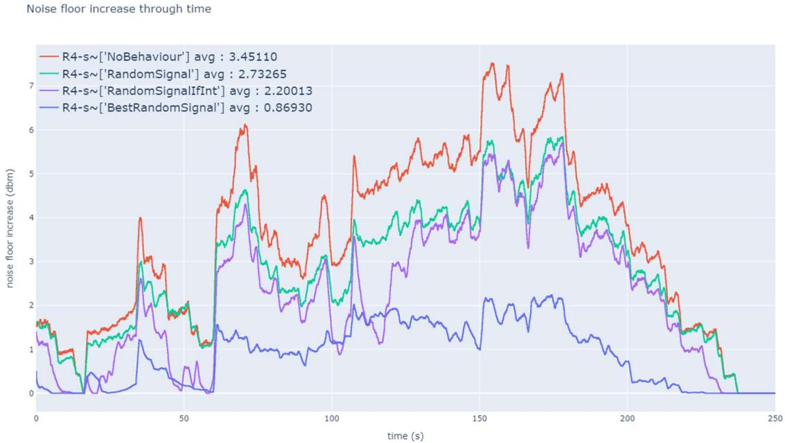
**Figure A1 – Average noise floor increase for radars on a 3km highway, 10 vehicles simulation**
