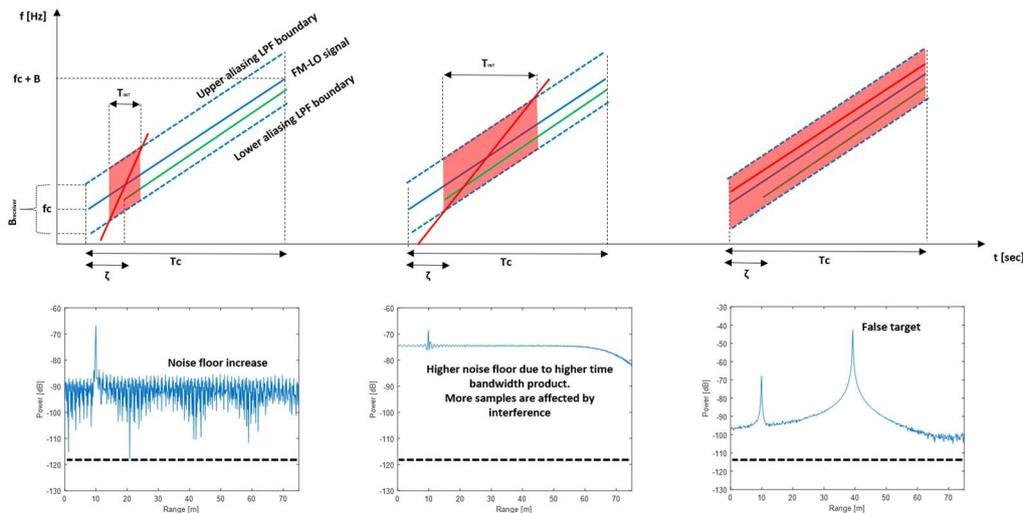
**Figure 2 – Effects of interference.** From left to right: (1) The interferer in red has a low correlation with the victim in blue, leading to a relatively small increase of the noise floor as few samples are affected. (2) As the correlation increases, the noise floor increases even more, leading to a potential blindness of the radar. (3) In the case of perfect correlation, the interference can be interpreted as a target as it resembles an echo of the blue signal
