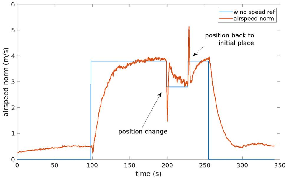
**Figure 14.** Evolution of the airspeed estimated from onboard filter and the reference wind speed.
