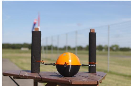
**Figure 2.** Quadrotor with custom spherical body shape.
