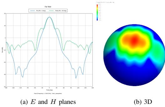
Fig. 7. Radiation pattern (dB) of the horn antenna.
