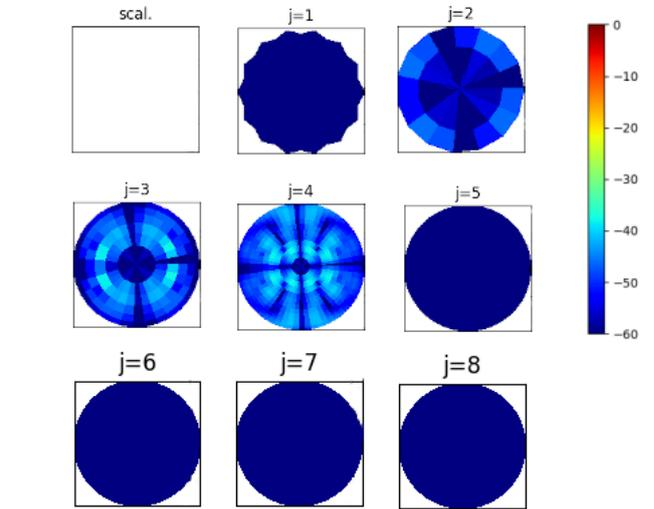
Fig. 8. Wavelet coefficients associated with the scaling function and the different wavelet levels for the horn antenna (dB).
