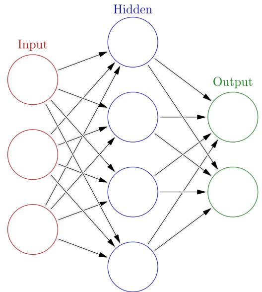
Fig. 3: Example of the structure of a dense neural network.
