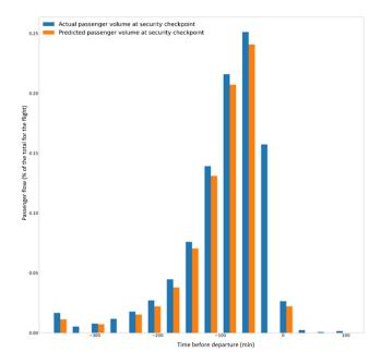
Fig. 7: Predicted mean passenger flow on an individual flight using Dense Neural Network.
