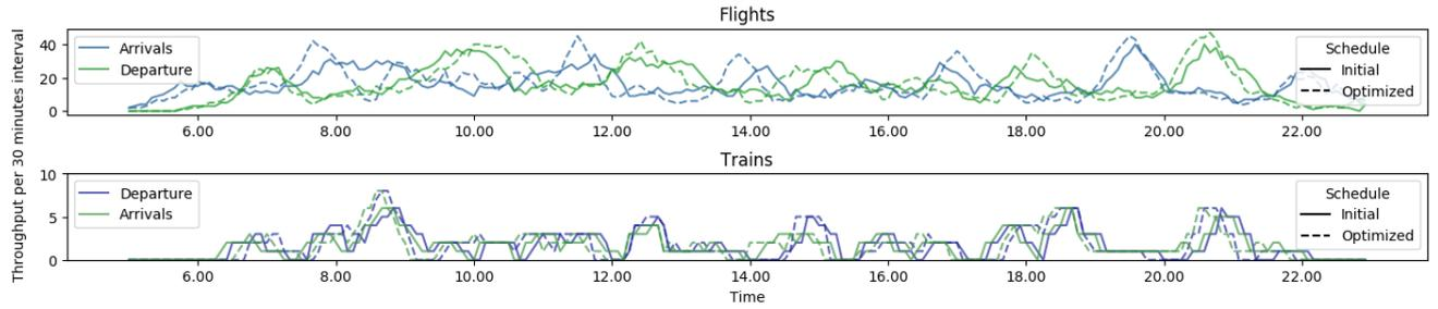
Fig. 5: Flights and trains arrival and departure throughput at CDG before and after optimization.
