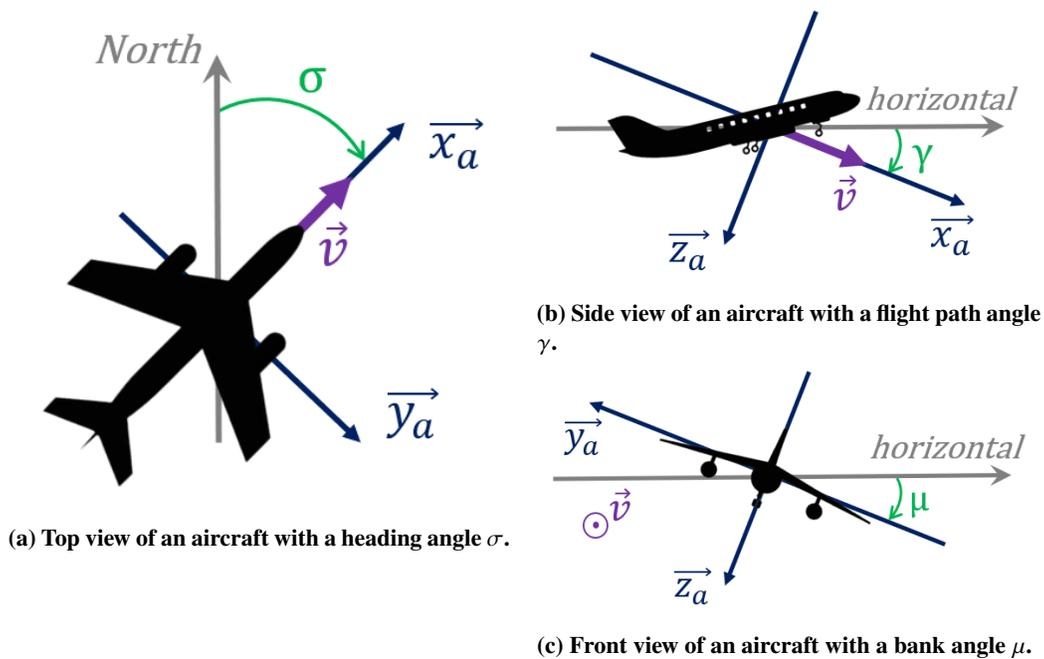
**Fig. 4** The aerodynamic frame  $(\vec{x}_a, \vec{y}_a, \vec{z}_a)$ . The frame origin is at the aircraft center of gravity, and the velocity vector  $\vec{v}$  (the aircraft true airspeed) is along  $\vec{x}_a$ .
