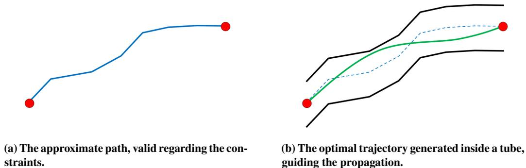
**Fig. 24 Building of a *guiding tube*.**
