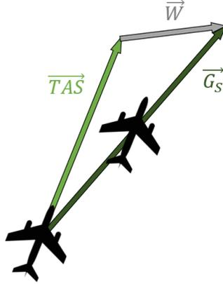
**Fig. 20** The Wind Triangle graphically represents the relationships among velocity vectors used for air navigation. As the true airspeed  $\vec{TAS}$  gives the heading of the aircraft, the ground speed  $\vec{G}_S$  provides the trajectory of the aircraft (relatively to the ground).
