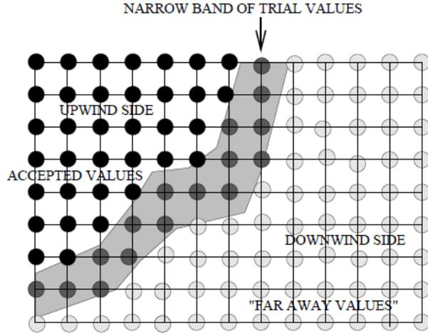
**Fig. 2** Upwind construction of accepted values [13, Fig. 14]. In the narrow band of trial values (*Close* in Alg. 1), the Eikonal equation is solved. The front propagates from accepted values (*Alive* in Alg. 1) towards "far away" values (*Far* in Alg. 1).
