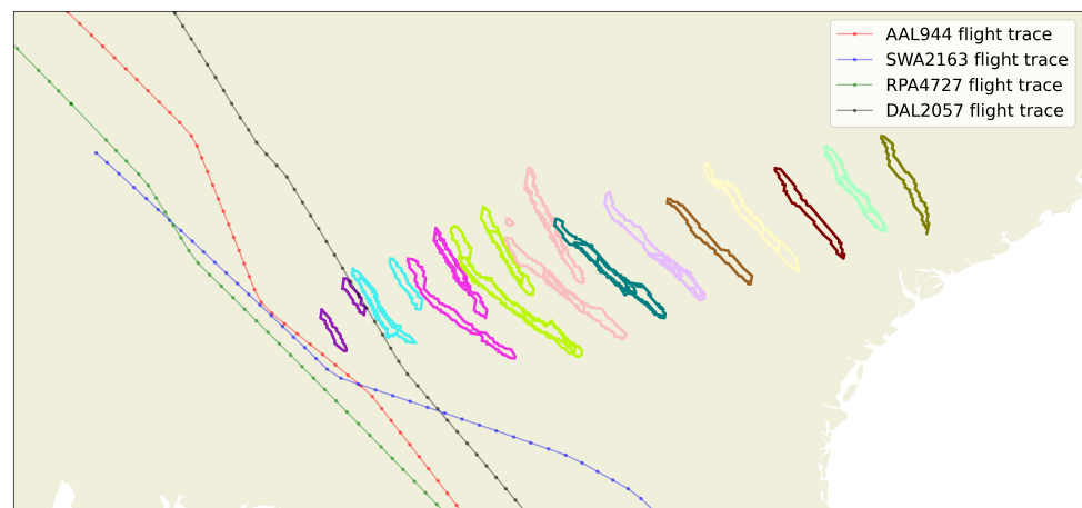
Figure 17. The situation at the beginning of the illustration example. Several polygons are detected on successive frames, and four flights flew in the area moments before the first polygons were detected.
