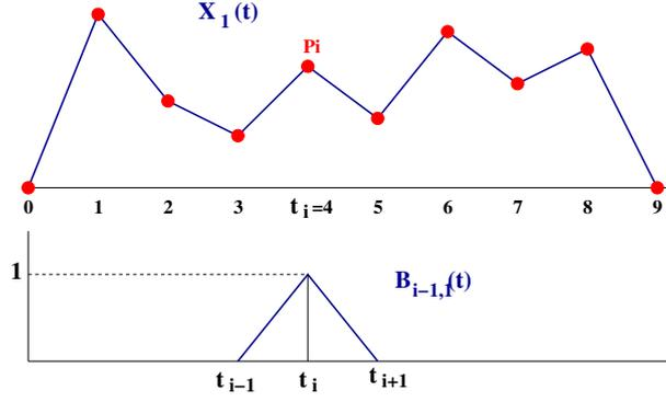
Figure 4.11: Uniform B-Splines of Degree One
