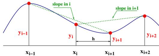
Figure 4.6: Piecewise cubic interpolation. The derivative at point  $x_i$  is given by line joining the point  $(x_{i-1}, y_{i-1})$  and  $(x_{i+1}, y_{i+1})$ . Between two points, a cubic polynomial is fitted. The term  $h$  represents the distance two consecutive points.
