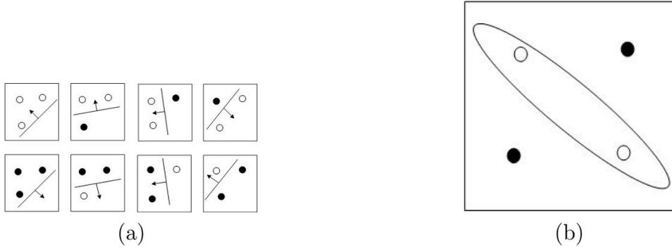
Figure 2.1: A linearly separable case and a non-linearly separable case. (a) the class of separating hyperplanes can shatter set of 3 points in  $\mathbb{R}^2$ . (b) the class of separating hyperplanes can not shatter set of 4 points in  $\mathbb{R}^2$ .
