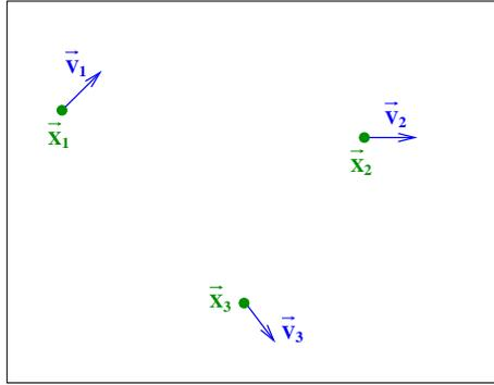
Figure 4.22: Radar captures associated with three aircraft
