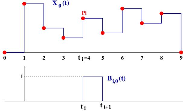
Figure 4.10: Uniform B-Splines of Degree Zero
