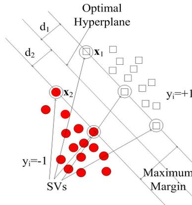
Figure 2.3: The Optimal Separating Hyperplane and Support vectors
