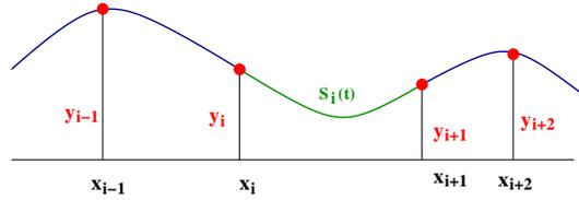
Figure 4.7: Cubic Spline Interpolation.
